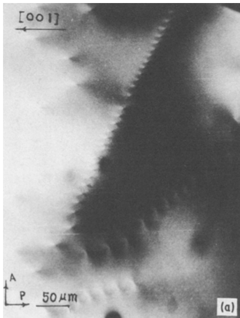
Figure 9 The effect of annealing on two rows of dislocations composed of Burgers' vectors \mathbf{b} = \frac{1}{2}[111] and [001] respectively: (a) before annealing the \mathbf{b} vector was deviated from the normal vector \mathbf{n} ; (b) after annealing at 700^\circ\text{C} for 7 h the normal of subboundaries line up parallel to the Burgers' vectors.
