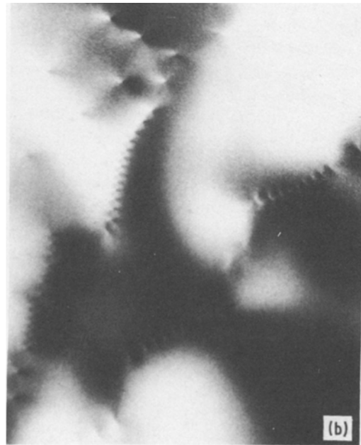
Figure 9 The effect of annealing on two rows of dislocations composed of Burgers' vectors \mathbf{b} = \frac{1}{2}[111] and [001] respectively: (a) before annealing the \mathbf{b} vector was deviated from the normal vector \mathbf{n} ; (b) after annealing at 700^\circ\text{C} for 7 h the normal of subboundaries line up parallel to the Burgers' vectors.
